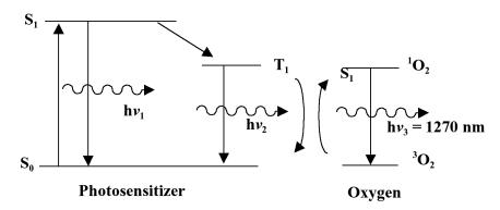
Figure 1b. The production of singlet oxygen from a photosensitizer.
